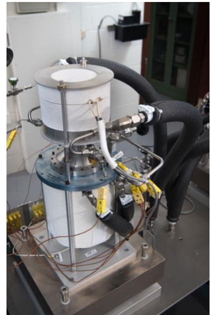
Figure 17. Infinia endurance test engine in operation at NASA GRC
