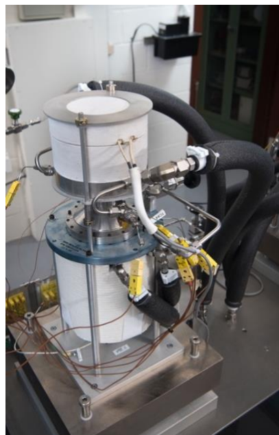
Figure 17. Infinia endurance test engine in operation at NASA GRC
